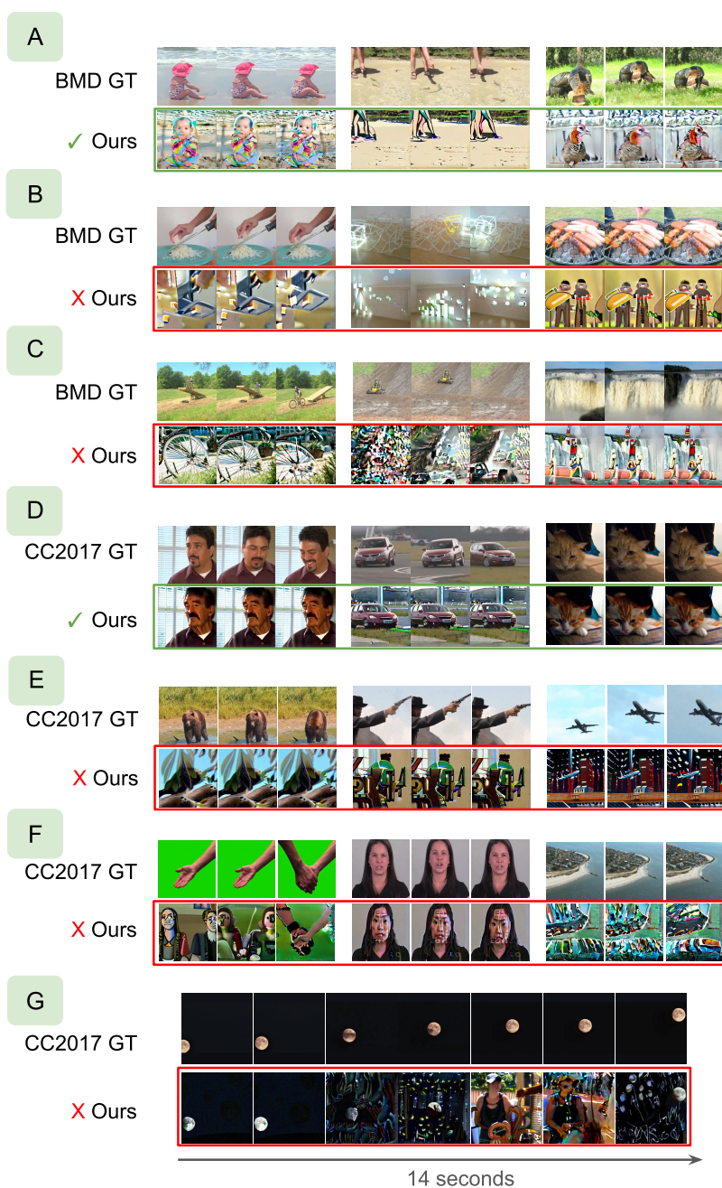
Fig. 4: Success and failure cases of reconstructions. A) Additional success cases from BMD. B) Additional failure cases from BMD. C) Specific failure cases from BMD exemplifying semantic dominance (left), high frequency noise (middle), and superposition of indiscernible shapes onto correct reconstruction (right). D) Additional success cases of CC2017. E) Additional CC2017 failure cases. F) Failure cases on CC2017 exemplifying semantic dominance (left), poor facial reconstruction (middle), high frequency noise (right). G) CC2017 failure case: Sudden failure to reconstruct video despite showing previous success in the segment.
